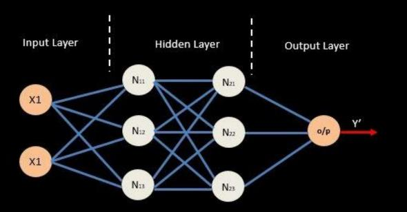
• The simplest form of neural networks where input data travels in one direction only, passing through artificial neural nodes and exiting through output nodes. Where hidden layers may or may not be present, input and output layers are present there. Based on this, they can be further classified as a single-layered or multi-layered feed-forward neural network.
